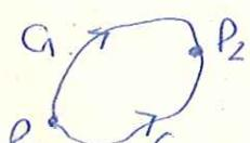
$$= \int_{C_1} \vec{F} \cdot d\vec{r} - \int_{C_2} \vec{F} \cdot d\vec{r} = 0 \rightarrow \boxed{\int_{C_1} \vec{F} \cdot d\vec{r} = \int_{C_2} \vec{F} \cdot d\vec{r}}$$
