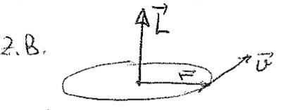
$\frac{d}{dt}(\vec{r} \times \vec{p}) = \dot{\vec{r}} \times \vec{p} + \vec{r} \times \dot{\vec{p}}$
