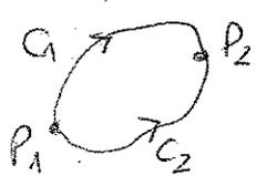
$$= \int_{C_1} \vec{F} \cdot d\vec{r} - \int_{C_2} \vec{F} \cdot d\vec{r} = 0 \rightarrow \boxed{\int_{C_1} \vec{F} \cdot d\vec{r} = \int_{C_2} \vec{F} \cdot d\vec{r}}$$
