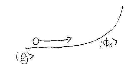
There's other form of constructing atomic mirror, namely the so-called magnetic mirror. A sheet of spatially alternating currents produces a magnetic field whose magnitude decreases exponentially when going out from the surface. The corresponding Zeeman effect is hence inhomogeneous. In this way an atom with a magnetic moment antiparallel to the magnetic field experiences a repulsive potential. So again a mirror.
