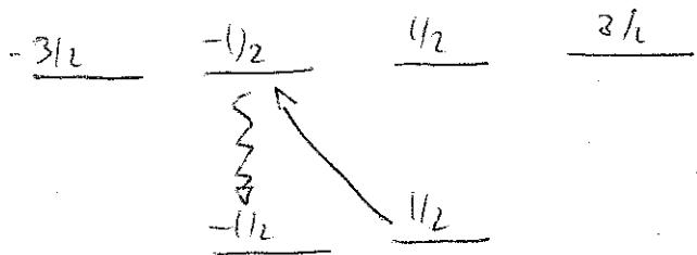
The transference rate from  $+1/2$  to  $-1/2$  is hence proportional to  $|S_{-}(z)|^2 \propto \cos^2(kz)$ , which is hence maximal for  $z=0, \lambda/2, \dots$  where the light is purely  $\sigma-$ , and it's zero for  $z=\lambda/4, 3\lambda/4$  where the light is purely  $\sigma+$ . One may actually write the transfer rate  $\gamma_{+-}(z) = \gamma \cos^2(kz)$
