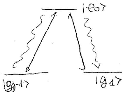
$$\hat{H}_{AL} = \frac{\hbar\Omega}{2\sqrt{2}} [1e_0\langle g_1 | e^{-ikz} - 1e_0\langle g_{-1} | e^{ikz}] e^{-iwt} + \text{H.C.}$$
