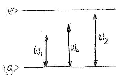
Therefore the atom absorbs with higher probability the photon ②, i.e. the counterpropagating photon. The atomic velocity is then reduced
