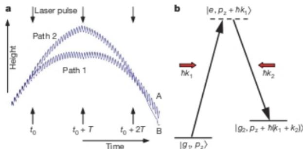
**Figure 2:** Atom interferometer and 2-photon Raman beam-splitter (Fig. 1 of Müller *et al.*). If  $k_1 := \|\vec{k}_1\| > k_2 := \|\vec{k}_2\|$ , then the transition  $g_1 \rightarrow g_2$  is accompanied by a four-momentum change of  $\Delta p = \hbar(\vec{k}_1 - \vec{k}_2, \omega_1 - \omega_2)$ , the transition  $g_2 \rightarrow g_1$  by  $-\Delta p$ .
